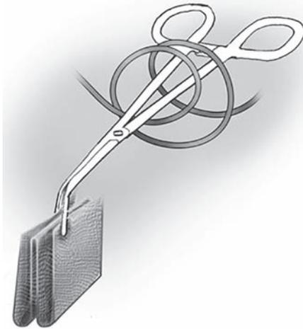
Fig. 13: Capacitance due to wrapping of monopolar electrode around artery forceps
