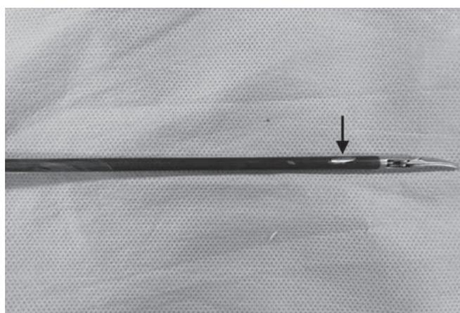
Fig. 9: Break in the insulation of monopolar scissor
