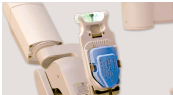
Fig. 51: Light-emitting diode (LED) blinking alternately white and green indicating activation of guided tool change.
