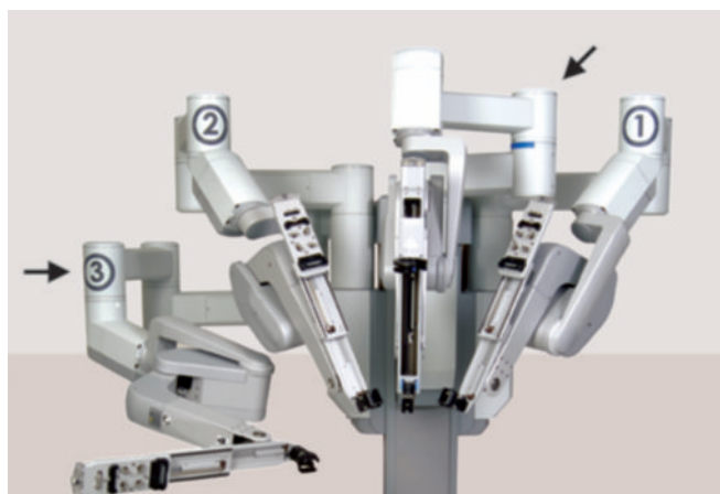
Fig. 35: Camera arm setup joint #2 facing opposite instrument arm 3 (arrow).
