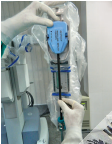
Fig. 47: Sliding the instrument into sterile adaptor on the instrument arm.
