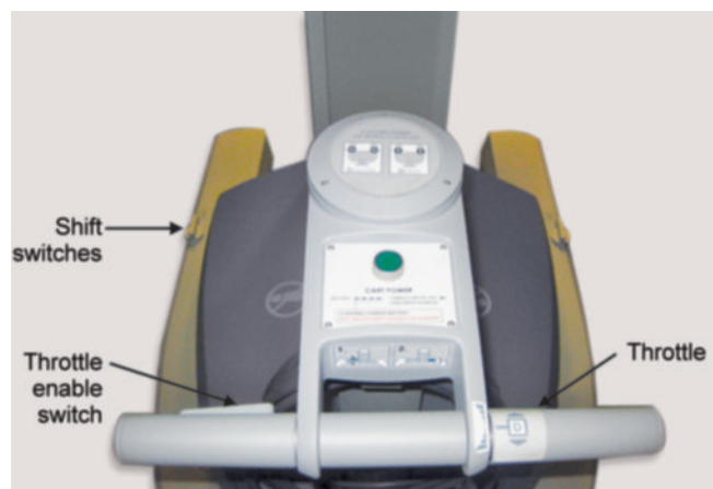
Fig. 22: Location of throttle, throttle enable switch, and shift switches.
